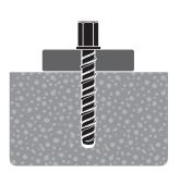
Continue to tighten the anchor until flanged head is firmly seated against fixture.
