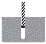
With the correct diameter drill bit, drill a hole to a depth of at least one diameter of the anchor deeper than the required embedment.
